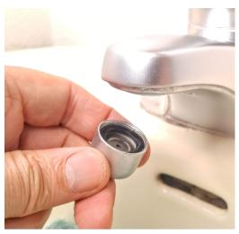
Faucet aerators mix air into the water stream to reduce the gallons per minute flow, saving you water and money. For bathroom faucets, choose a 1.5 or 1.0 gallon per minute (gpm) aerator. In the kitchen, where you fill pots with water, a 2 gpm aerator will be more effective.
