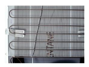
We recommend cleaning the refrigerator condenser coils at least once a year. In most cases, the refrigerator's condenser coils can be found on the back lower part of the refrigerator. Please follow the instructions below to clean the refrigerator condenser coils.
